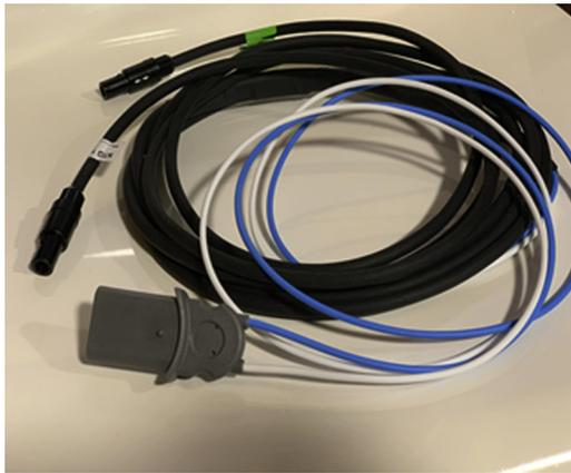
Standard outlet cords of a biphasic defibrillator (**blue and white**) were manually wired to 2 proprietary cables (**black**), and the latter cables were connected to each standard ablation catheter in bipolar fashion.
